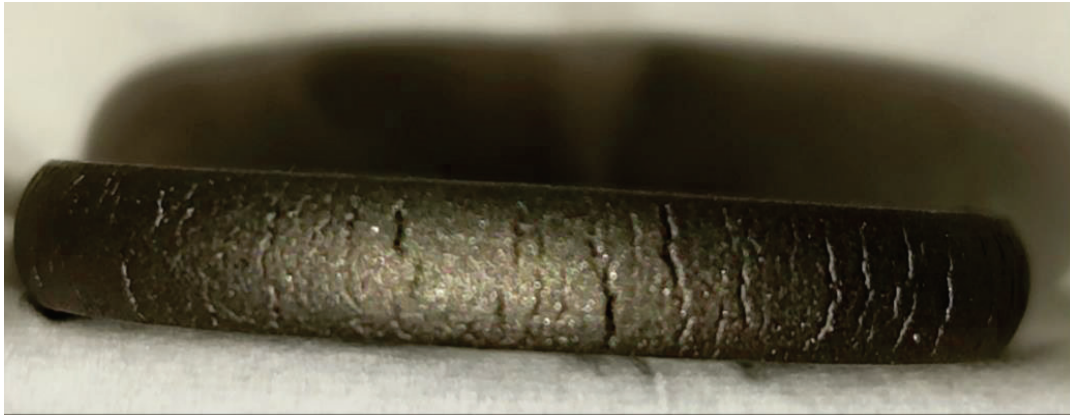
Fig. 5. Cracks on the lateral surface of the ring specimen lubricated with WL1.
