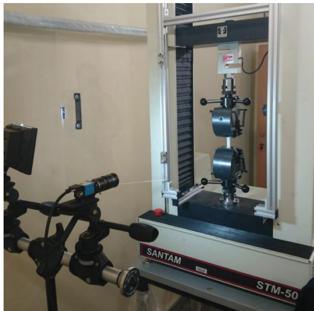
Fig. 3. Schematic of the experimental setup used for tensile testing and digital image correlation (DIC)
