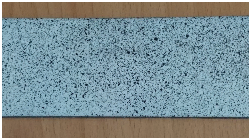
Fig. 2. Speckle pattern generated on the specimen surface for DIC analysis
