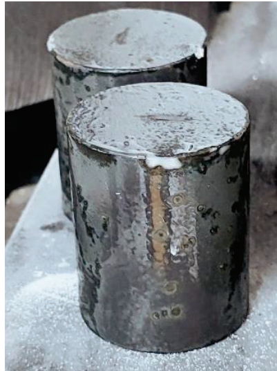
Fig. 2: Final section coated with WL1 lubricant for adhesion testing.
