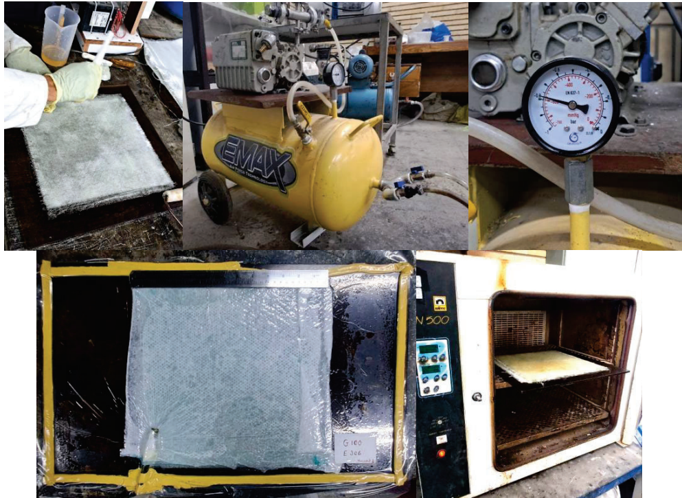
Figure 4. The process of making composites (Part II); includes the steps of finalizing the layers and removing excess resin, closing the vacuum bag and applying vacuum pressure for CR306 (-0.8 bar), and thermal curing in oven for ER 440 (150°C).
